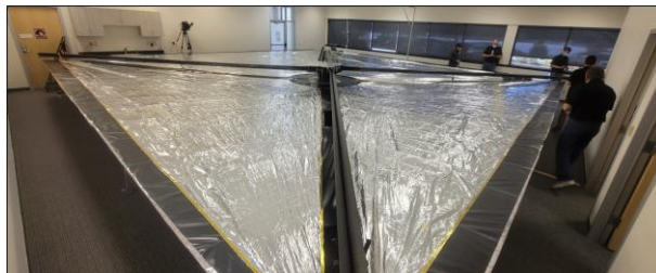
Fig. 4. Quarter-scale sail deployment test.
